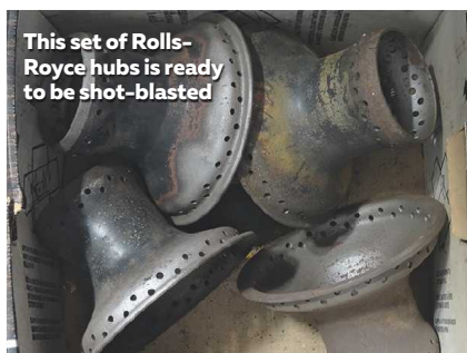
Some Rolls-Royce hub designs are complex and would be expensive to reproduce
