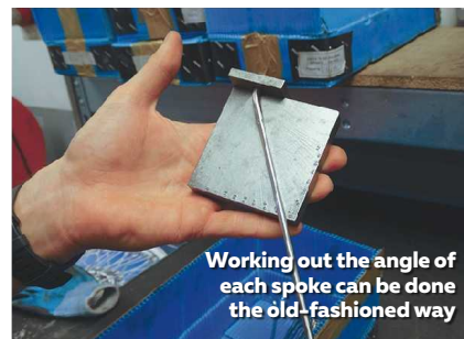
Each hole has to be at exactly the right angle for that particular spoke
