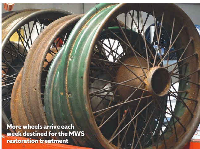
This set of Rolls-Royce hubs is ready to be shot-blasted
